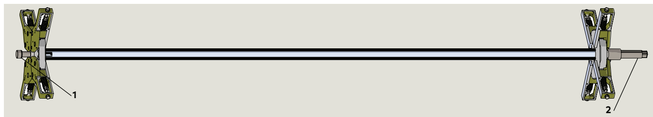
Fig. 16.2.1 RS6060-001, 4 wing steel shaft assembly
